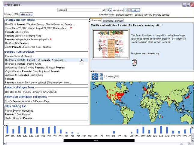
Figure 1: Snapshot of the system. The panel on the top left shows the distinct clusters associated with the query “peanuts”. The top right panel displays the summary of a specific page selected by the user. Spatial characteristics of the data are displayed on an interactive map. An interactive timeline at the bottom displays the temporal distribution of the results. All the modules are reflectively interlinked.
